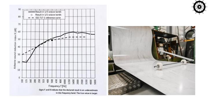
Bend test: The panel is strong enough, no deflection at 135 kg. The product is protected worldwide with different patents.
